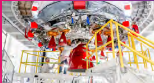
Technicians working on the European Service Module, which provides power and propulsion to the Orion spacecraft carrying the astronauts to lunar orbit in the Artemis II mission.
